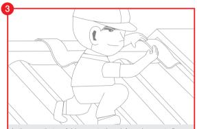
In the area that roof ridge meets the reinforced concrete flange, install the round ridge to line of RC flange. Leave gap between round ridge and RC flange about 3 cm. Slightly fold the edge of SCG Flashing and insert under RC flange, compress SCG Flashing to perfectly adhere with round ridge and tile panel.
